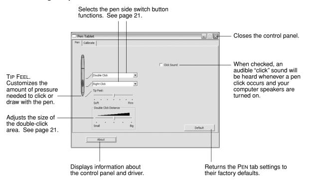
**Hint:** To create broad brush strokes or to click with a light touch, use a soft tip setting. A soft setting provides a wider range of pressure values with most pressure-sensitive applications. In some applications, a soft pressure setting can make the pen overreact – any small press on the pen is magnified on the screen. If you experience this, try a firmer tip setting.
